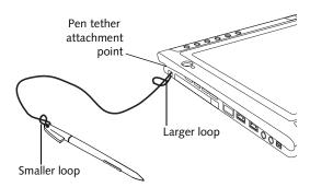
Figure 2-1 Installing a Pen Tether
